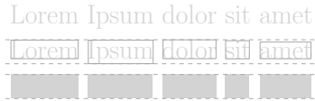
Figure 5: Words' bounding boxes are normalized in height. This allows the user to easily select (or draw over) them, but also to find the gesture context.
