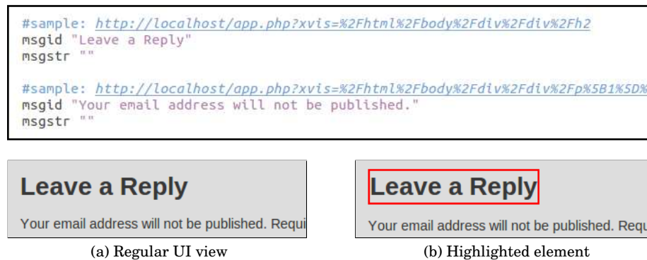
Fig. 8: Automatic PO generation augmented with visual context hints. Each resource string is attached a URL that provides translators with an example of the element containing such string.
