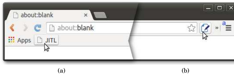
Fig. 6: Both the bookmarklet (a) and the browser extension (b) inject a single line of JavaScript code to the DOM so that the required libraries are automatically loaded.
