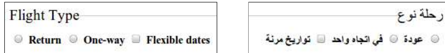
Fig. 4: JITL changes the text direction and UI layout according to the target language the user is localizing into.
