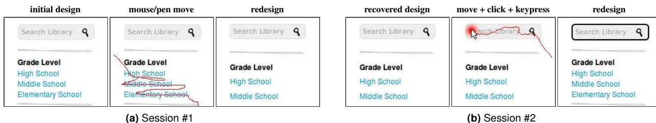
Figure 1: This adaptation technique is tightly coupled to the user interactions, but also delimited by the UI developer. In this example, the system is allowed to modify the border-width and border-color properties of the search box, and the padding-top property of the list items. In the first session (1a) the list is hovered, and hence the padding is increased accordingly. In the second session (1b) the previous redesign is recovered from the local database. Since this time the user does not interacted with the list items, the padding is therefore decreased.
