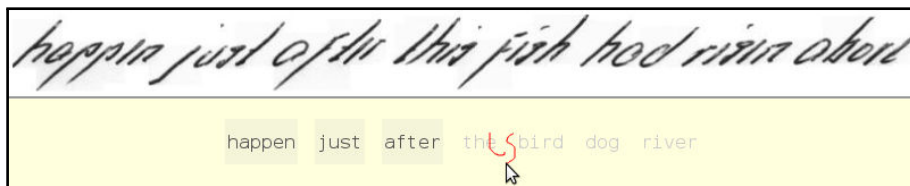
Figure 6.3: Interactive Handwritten Transcription prototype, an example of structured input. Some word-level editing operations that can be performed are substitution (shown in the image), insertion (6.2a), deletion (6.2b), or rejection (6.2c). In this example, the system assumes that the first 3 words plus the first 2 characters of the edited word are correct. This information is used to 1) decode the submitted pen strokes and 2) predict a suitable continuation of the implicitly validated segment: “ happen just after this fish ... ”. Prototype available at http://cat.iti.upv.es/ih/ .
