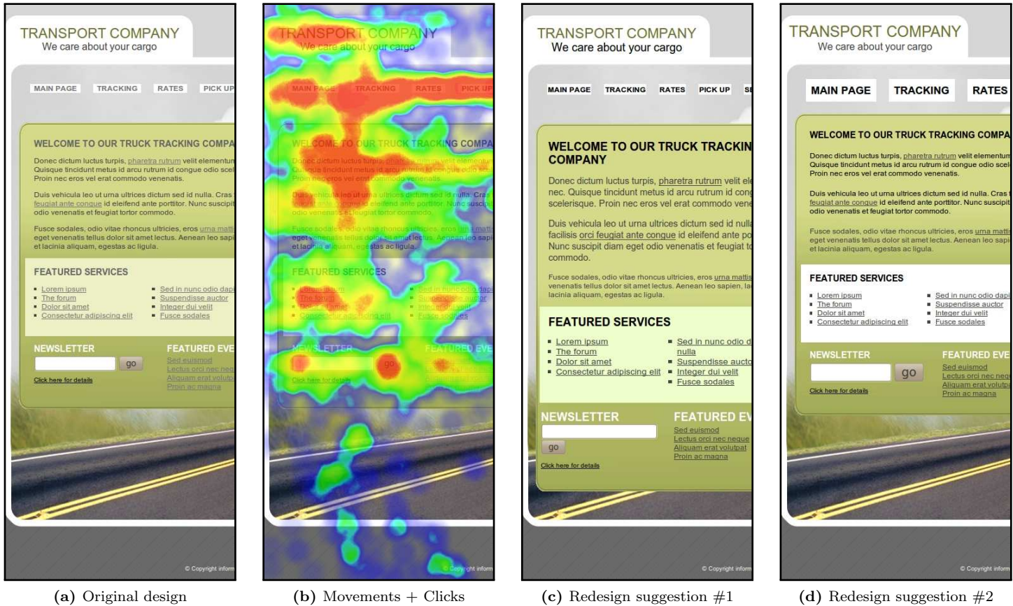
Figure 5.9: Redesign examples produced by ACE, taking into account multiple interaction logs and overriding a few CSS rules.
