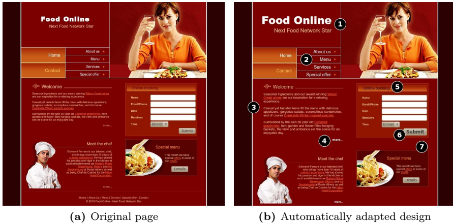
Figure 5.1: An example of website design modifications. Changed parts are numbered in Figure 5.1b. ① headline text: font-size, padding-top; ② navigation menu: font-size; ③ welcome paragraphs: font-size; ④ ‘read more’ links: color; ⑤ ‘online booking’ heading: color; ⑥ submit button: font-weight; and ⑦ ‘special menu’ div: margin-top.
