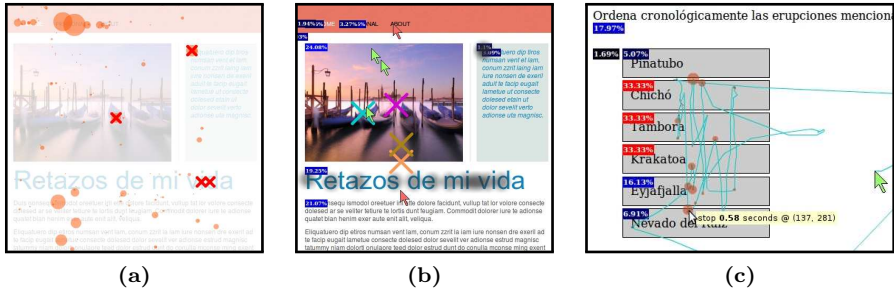
Figure 2.5: Combining visualization possibilities. [2.5a] Displaying hesitations (circles) and clicks (small crosses). [2.5b] Displaying entry/Exit coordinates (cursor bitmaps), motion centroids (big crosses), drag&drop activity (shaded fog), and interacted DOM elements. [2.5c] Analyzing a decision process; the user rearranged items in a list. Small circles represent dwell times. Hovered DOM elements are labeled based on frequency (percentage of browsing time), including a blue color gradient (100% blue: most hovered items). The same scheme is used to analyze clicked items, but using the red palette.
